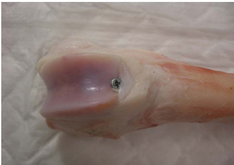
Fig.2. A screw was inserted dorsal to the trochlea ossis femori at the distal end of the femur and used as a reference point in the pQCT measurements.
