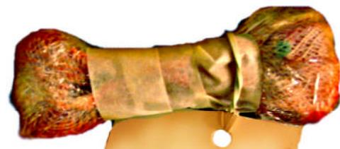
**Figure 6.** The bones were moistened with ringer solution and covered with gauze bandage and polythene.
