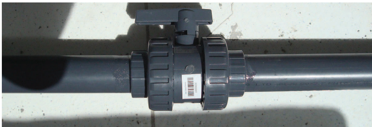
Figure A2. The joint between two PVC tube sections, notice the lever of the valve on top. Joel Segersten, Uppsala University 2008.
