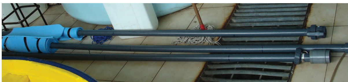
Figure A3 The three sections of the dissembled sediment sampler. Each section measures ~3 meters, the module for Willner core attachment is visible in the lower right corner and the metal ring for fitting the rope can be seen just above the connection module. The floating device is visible to the left. Joel Segersten, Uppsala University 2008.
