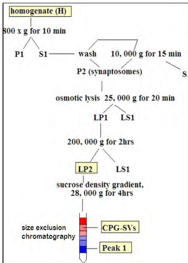
Figure 3. A flow chart depicting the procedure of purifying 'Controlled Pored Glass synaptic vesicles' (CPG-SVs) from a homogenate of rat brain tissue. The yellow boxes indicate the fractions used in this study: the Homogenate (H), Lysed Pellet 2 (LP2), the purified synaptic vesicles (CPG-SVs) and Peak 1 (I).
