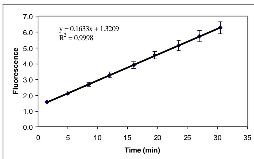
**Figure 9.** Progress curve of MMP-2 catalytic domain activity in a CD-microlaboratory. The reaction proceeds for at least 30 minutes in the CD (CDE6Q). The figure shows the increase in fluorescence with reaction time in the highest tested concentration of the catalytic domain (20 nM). Fluorescence was measured off-line with a PMT setting of 0.35. CV(n=3) was 4-7 %. The assay was performed with 10  $\mu$ M substrate.
