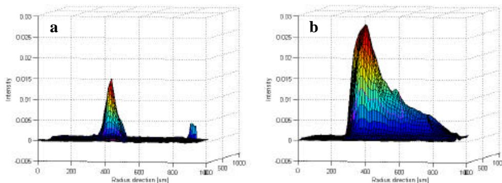
**Figure 22.** Sandwich immunoassay of proMMP-2 downstream of a reaction chamber in a CD-microlaboratory. Fluorescence distribution in columns loaded with 8.33 nM (75nl) proMMP-2, 2000 nM (0.3 mg/ml) of capturing antibody and 300 nM detecting antibody. a) 2  $\mu$ M (75 nl) of substrate had been loaded through the common distribution channel, b) PBS-Tween was applied instead of substrate.
