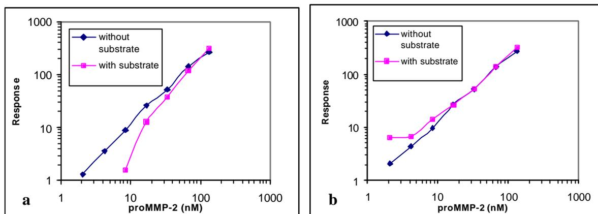
**Figure 21.** Sandwich immunoassay of proMMP-2 downstream of a reaction chamber in a CD-microlaboratory. ProMMP-2 quantified with 2000 nM capturing antibody MAB 903 and 300 nM detecting antibody AF902 (3.09 mol Alexa™ 647/mol AF 902) both in presence and absence of 1  $\mu$ M FRET substrate. One sample was analysed at each concentration. a) background has been subtracted from the values, b) no background subtraction has been made.
