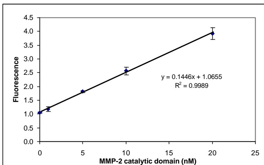
**Figure 7.** Enzyme activity of MMP-2 catalytic domain in a CD-microlaboratory. The protease (75 nL, 1-20 nM) was mixed with FRET peptide substrate (75 nL, 10  $\mu$ M) in CDE6Q and the catalytic activity was assayed after 16 minutes through off-line fluorescence detection with a photo multiplier tube (PMT) setting of 0.35.
