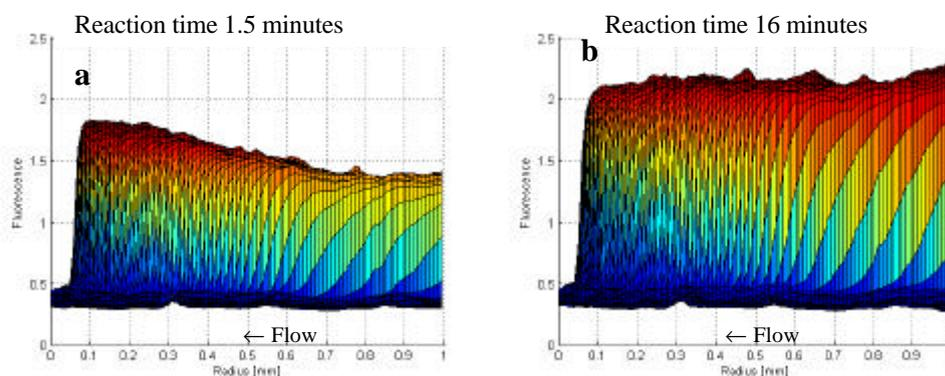
**Figure 8.** Enzyme activity assay with MMP-2 catalytic domain in a CD microlaboratory. Fluorescence distribution in reaction chambers containing 5 nM MMP-2 catalytic domain. Both pictures show the same microstructure; a) after 1.5 minutes of reaction and b) after 16 minutes. Initially substrate is enriched at the bottom of the basin, but after 16 minutes of incubation the solutions are homogeneous with flat fluorescence profiles.
