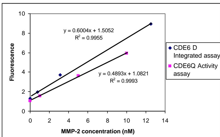
**Figure 20.** Enzyme activity of MMP-2 in different CD microstructures. In the enzymatic assay in CDE6 Q (■) active MMP-2 was run in triplicates in buffer containing 0.025% Brij-35. In the integrated assay in CDE6 D (◆) the enzyme was run in duplicates in buffer with 1% BSA and resulted in detection limits of 0.10 nM. The activity appeared to differ with a factor of 1.2 when analysed in the different structures. Fluorescence was recorded off-line with PMT settings of 0.35.
