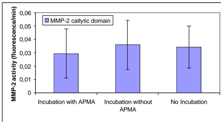
**Figure 11.** Enzyme activity of the MMP-2 catalytic domain after incubation at 37 °C. The enzyme activity in samples of the catalytic domain incubated for 2 hours at 37 °C with or without p-aminophenylmercuric acetate (6  $\mu$ M) was within experimental error the same as in non-incubated samples of the catalytic domain. The catalytic domain (10 nM) was assayed in triplicates with 10  $\mu$ M substrate in CDE6 Q.
