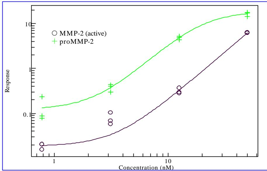
**Figure 17.** Sandwich immunoassay of MMP-2 in a CD-microlaboratory. ProMMP-2 (+) and active MMP-2 (○) quantified in CDBA2 with 533 nM (0.08 mg/ml) capturing antibody and 100 nM fluorophore conjugated antibody (degree of labelling: 3.09 mol Alexa™647 /mol AF 902). PMT settings were 1% and background fluorescence was not subtracted from the responses.
