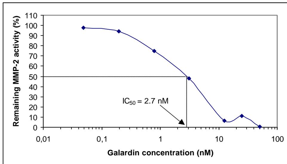
**Figure 13.** Inhibition of MMP-2 by galardin. Galardin was mixed with substrate (10  $\mu$ M) and activity was determined through a homogeneous assay in CDE6 Q with MMP-2 (10 nM) added through the common channel.
