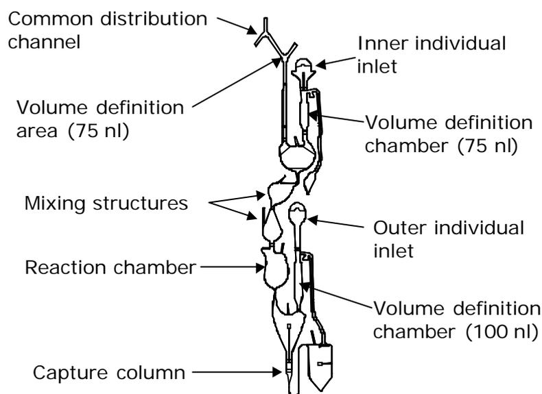
**Figure 6.** Design of the microstructure CDE6 D. The microstructure was used for performing integrated enzyme activity and quantification assays. The illustration was used with permission from Mats Inganäs at Gyros AB.
