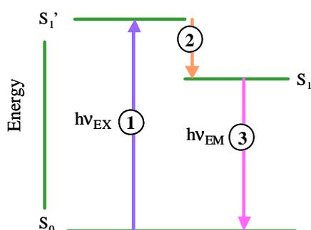
**Figure 3.** Principle of the molecular event of fluorescence (Jablonski diagram). Fluorescence occur in a three step process with 1) excitation, 2) loss of energy through vibration and 3) emission. The illustration was adapted from (Amersham Biosciences, 2002)
