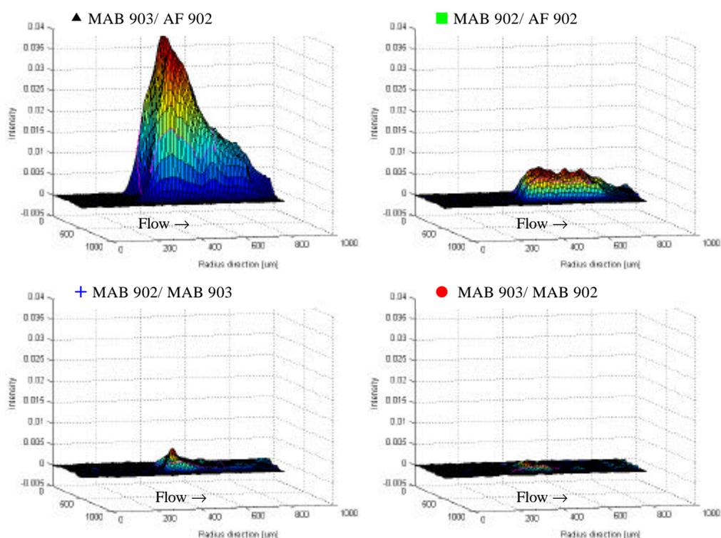
**Figure 16.** Evaluation of capturing and detecting antibody pairs. The fluorescence distribution in columns of CDBA2 loaded with 12.5 nM proMMP-2 and different antibody pairs. ▲ MAB 903 capturing / AF 902 detecting, ■ MAB 902 capturing / AF 902 detecting, + MAB 902 capturing / MAB 903 detecting, ● MAB 903 capturing / MAB 902 detecting.
