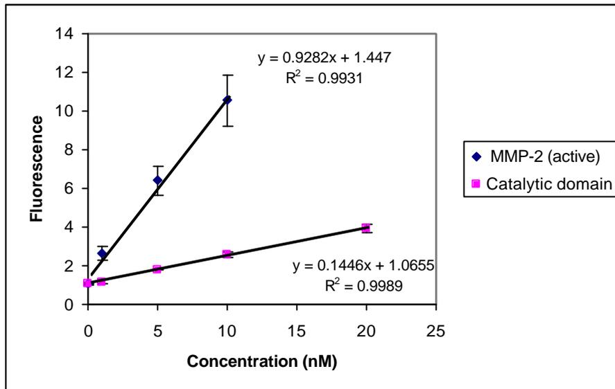
**Figure 12.** Enzyme activity of MMP-2 and the catalytic domain of MMP-2 in CD-microlaboratories. The various forms of the protease were assayed in triplicates with 10  $\mu$ M FRET substrate in CDE6Q, at different occasions. The activity of MMP-2 was approximately 6 times higher than that of the catalytic domain. The assay time was 16 minutes.
