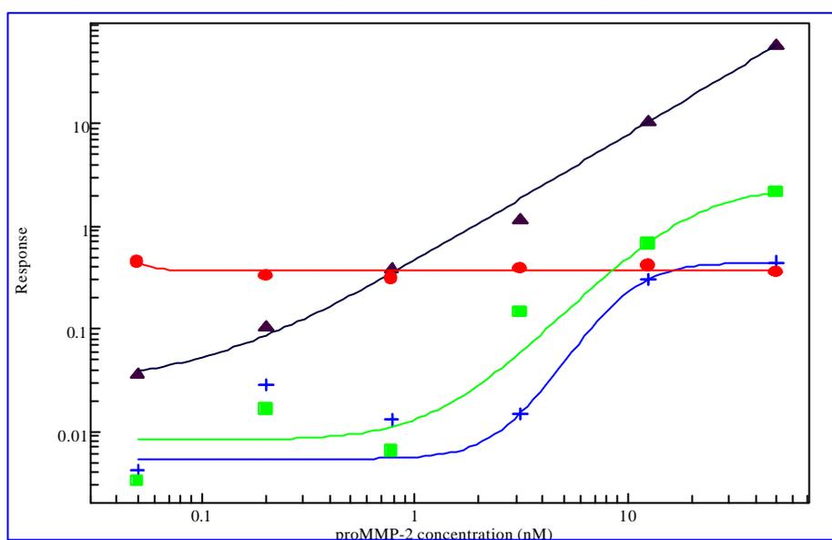
**Figure 15.** Evaluation of capturing and detecting antibody pairs. Four antibody pairs were assayed in parallel in CDBA2; ▲ MAB 903(monoclonal antibody)/AF 902 (polyclonal antibody), detection limit 0.4 nM; ●MAB 903 /MAB 902 (monoclonal antibody); +MAB 902/ MAB 903 and ■ MAB 902 /AF 902. The curves were generated from on-line fluorescence recordings with PMT settings of 5%.
