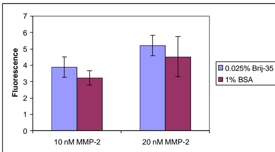
**Figure 14.** MMP-2 activity in the presence of protein. The fluorescence intensities obtained when performing an enzyme activity assay in buffer containing 1% (w/v) BSA were slightly lower, but within experimental error the same as in runs with Brij-35 buffer. All samples were run in triplicates in Q structures on the same CDE6. MMP-2 activity was analysed with 10  $\mu$ M substrate.
