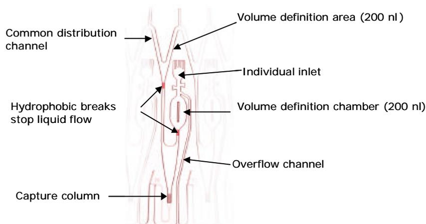
**Figure 2.** Illustration of the common features found in the microstructures on the CDs. This particular structure has an affinity column at the lower end and is used for sandwich immunoassays. The illustration was used with permission from Mats Inganäs at Gyros AB.
