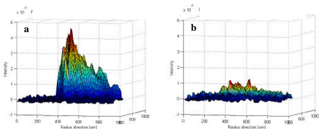
**Figure 19.** Sandwich immunoassay of proMMP-2 in a CD-microlaboratory. Fluorescence distribution in columns having 1000 nM (0.15 mg/ml) of capturing antibodies attached to the surface. a) 0.51 nM proMMP-2 and 145 nM of detection reagent and b) 0.78 nM proMMP-2 and 100 nM of detecting antibody.
