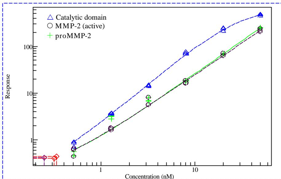
**Figure 18.** Sandwich immunoassay of MMP-2 in a CD-microlaboratory. ProMMP-2 (○), active MMP-2 (+) and the catalytic domain of MMP-2 (△) quantified in CDBA2 with 1000 nM (0.15 mg/ml) of capturing antibody MAB 903 and 145 nM of detecting polyclonal antibody AF 902 (degree of labelling: 3.09 mol Alexa™647 /mol AF 902). The detection limit was 0.3 nM for all MMP-2 forms. The curves were generated from detections with PMT settings of 5%.
