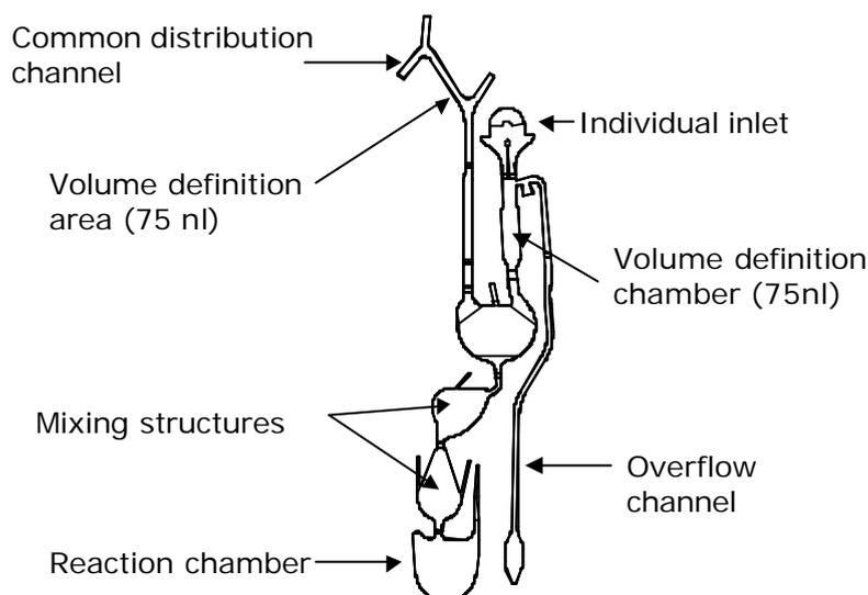
**Figure 4.** Design of microstructure CDE6 Q for enzyme activity assay. The illustration was used with permission from Mats Inganäs at Gyros AB.
