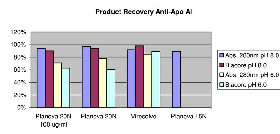
Figure 6. Product recovery from filtration trials using Anti-Apo AI. The protein concentration was 150 µg/ml, unless else is stated, and the filtrated volume was 10 ml.
