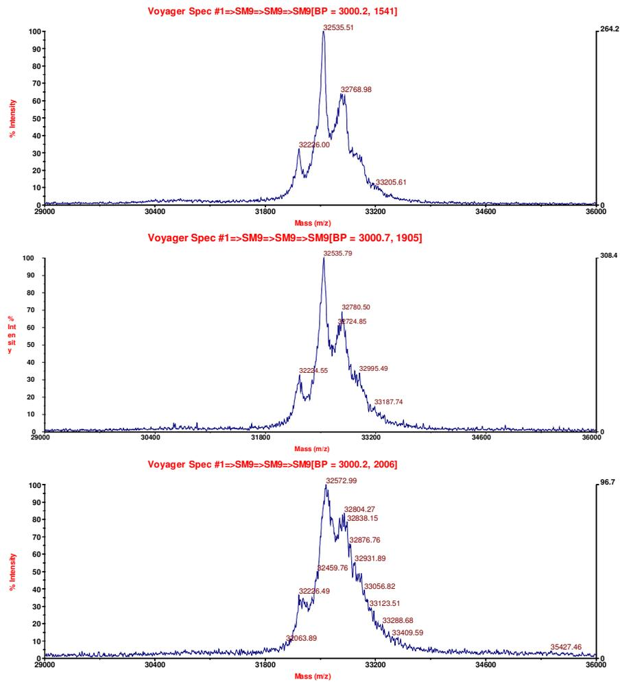
Figure 17. Mass spectra from MALDI-TOF analysis of PROTEIN Z. Top. Non-treated PROTEIN Z, Middle. Control-treated for 24 hours at 37°C, pH 5.0, Bottom. 5 mM IAA for 24 hours at 37°C, pH 5.0
