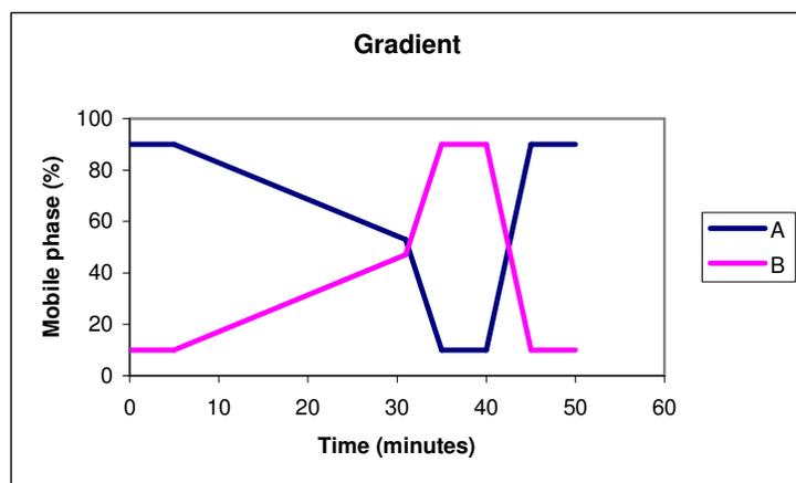
Figure 4. The gradient used in the RP-HPLC analysis.
