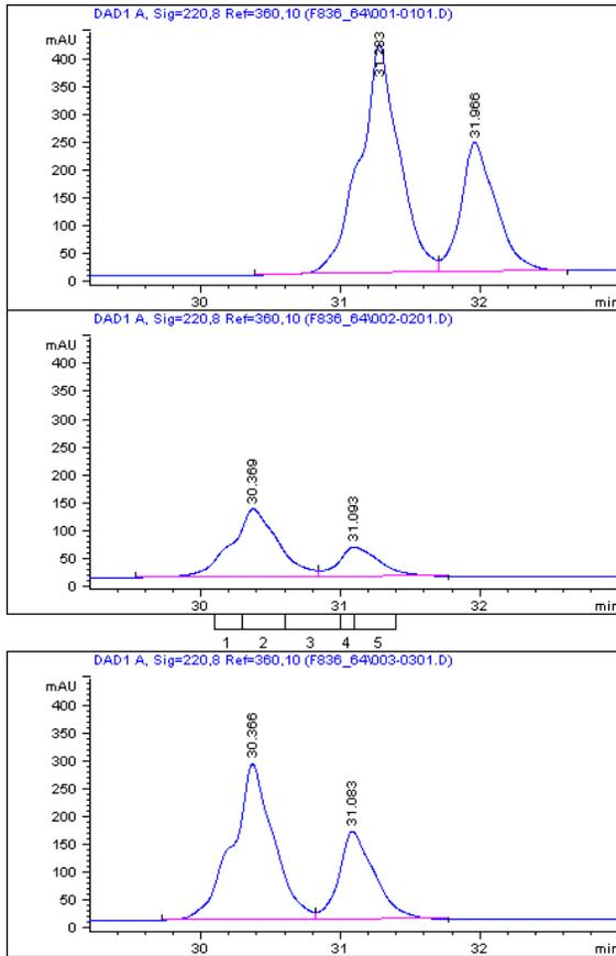
Figure 18. Chromatograms from RP-HPLC run with PROTEIN Z. Top: Non-treated PROTEIN Z. Middle: PROTEIN Z treated with 5 mM IAA for 24 hours at 37 °C and pH 5.0. Bottom: Control-treated PROTEIN Z, 24 hours at 37 °C and pH 5.0. Fractions, if collected, are marked under the respective chromatogram.
