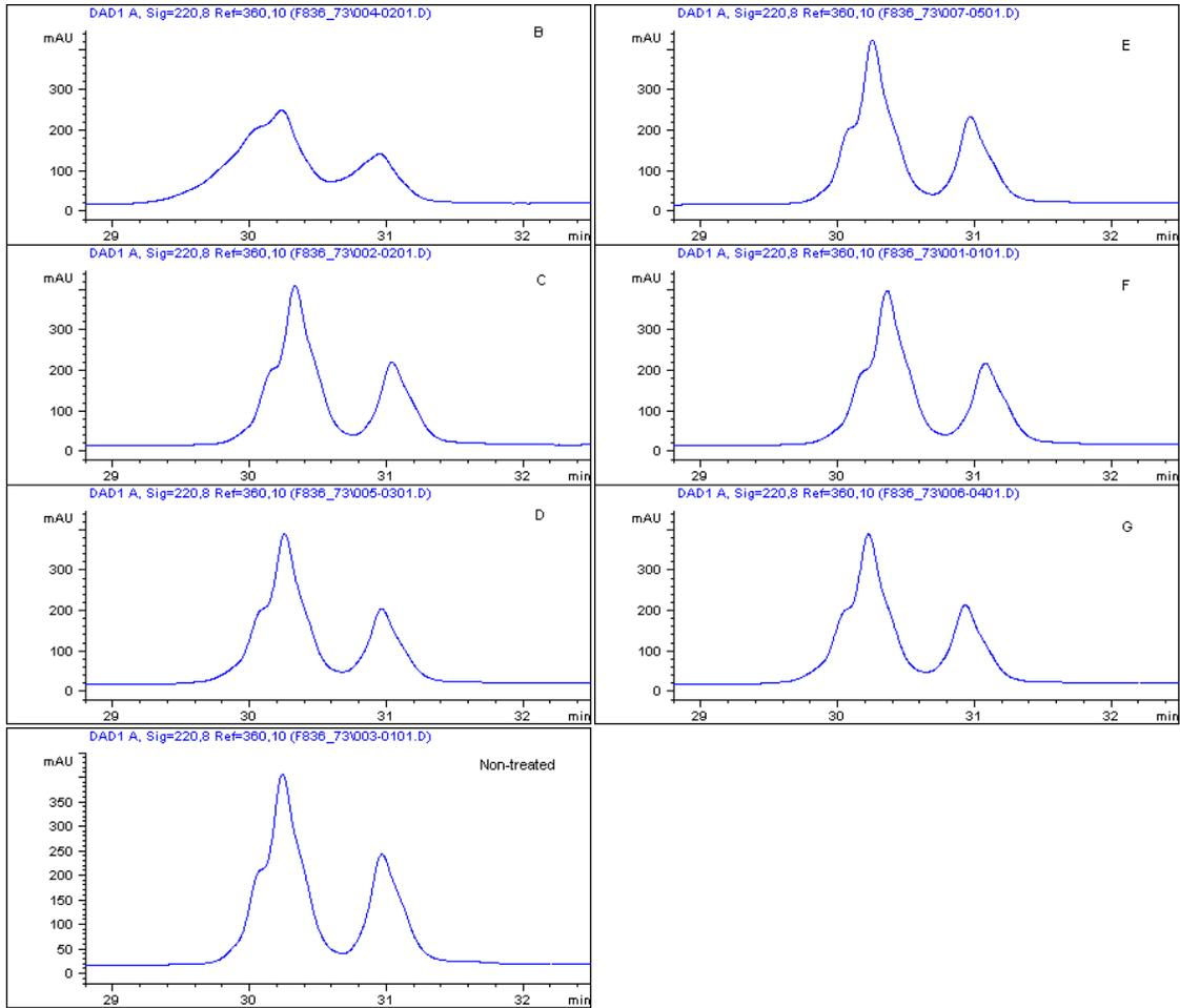
*Figure 13.* Chromatograms from RP-HPLC runs with PROTEIN Z. Samples B-G were treated according to table 4. B) 0.2% INACTINE for 24 hours at 37 °C and pH 6.0. Samples C, D, F and G were treated with 0.1 % INACTINE at pH 7.2, C) 24 hours at room temperature, D) 24 hours at 37 °C, E) Control-treated PROTEIN Z, 24 hours at 37 °C, F) 3 hours at 37 °C, G) 24 hours at room temperature, 50 mM NaCl. Non-treated sample was diluted in 50 mM Na-acetate, pH 5.0
