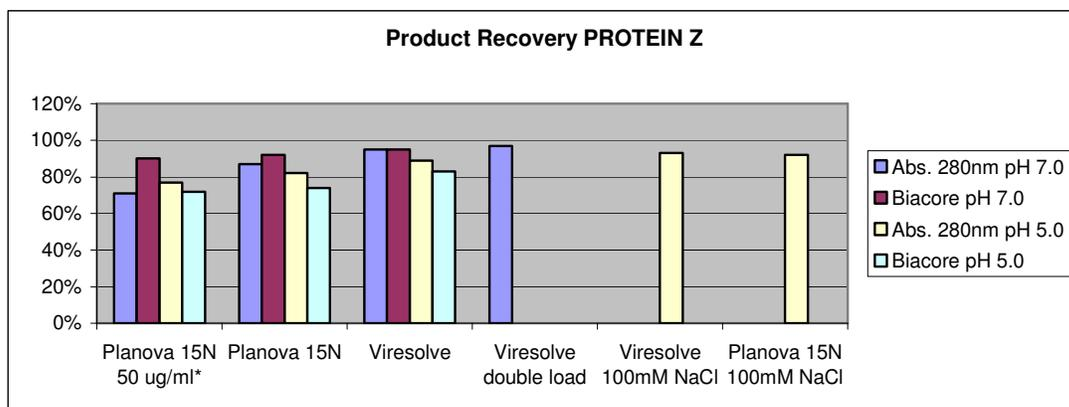
Figure 5. Product recovery from filtration trials with PROTEIN Z. Protein concentration was 150  $\mu\text{g/ml}$ , except for when else is stated, and filtrated volume was 15 ml. \*A280 was out of range ( $<0.1$  AU) and results may not be reliable.
