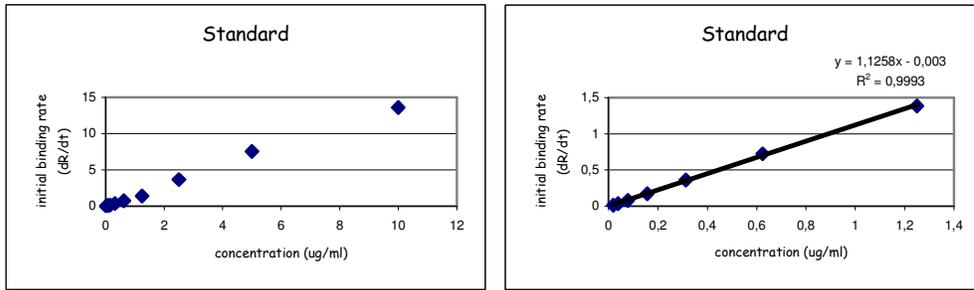
Figure 2. Example of a standard curve for Anti-Apo AI. The curve is only linear at low concentrations of analyte and the interval used for measurement is shown to the right.
