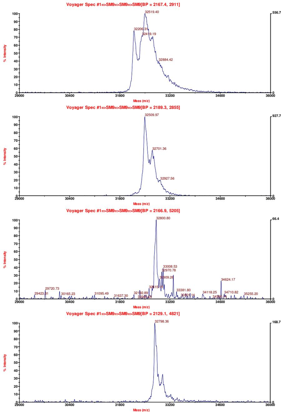
Figure 19. Mass spectra from MALDI-TOF analysis of RP-HPLC fractions of IAA-treated PROTEIN Z (see figure 18 middle). From top to bottom: fraction 1, fraction 2, fraction 4 and fraction 5. The signal was low for fractions four and five.
