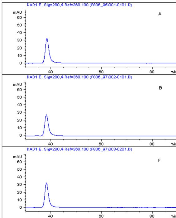
Figure 21. Chromatograms from SEC run with PROTEIN Z. Samples were treated according to table 7 and desalted on PD-10 columns. A) Control-treated PROTEIN Z, 24 hours at 37 °C. B) and F) were treated with 5 mM IAA at pH 5.0. B) 24 hours at 37 °C, F) 3 hours at 37 °C.
