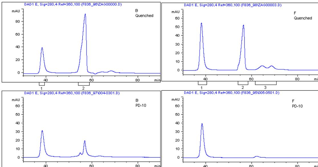
Figure 14. Chromatograms from SEC runs with PROTEIN Z. Samples were treated with INACTINE according to table 6. B) 0.2% INACTINE for 24 hours at 37 °C, pH 6.0, F) 0.1% INACTINE for 3 hours at 37 °C, pH 7.2. Fractions, if collected, are marked under respective chromatogram.
