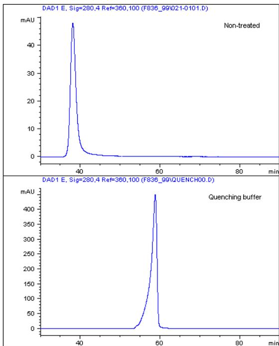
Figure 16. Chromatograms from SEC analysis. Top. Non-treated PROTEIN Z diluted in 50 mM Na-acetate, pH 5.0, Bottom. Quenching buffer (25 mM Phosphate buffer, 500 mM Sodiumthiosulphate, pH 7.0.) The chromatograms are scaled differently.
