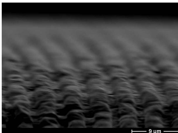
*Figure 10. Scanning electron micrograph of cut edge of PCL replica coated with <math><0.5 \mu\text{m}</math> layer of gold.*
