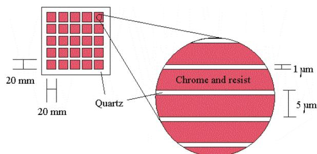
**Figure 9.** Quartz plate with inscribed chrome and resist mask with a period length of 5  $\mu\text{m}$ .
