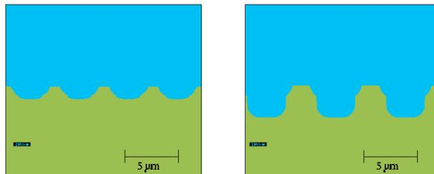
**Figure 8.** Structures simulated in 2Dinese. In (a) only isotropic, (b) both directional and isotropic etching used.
