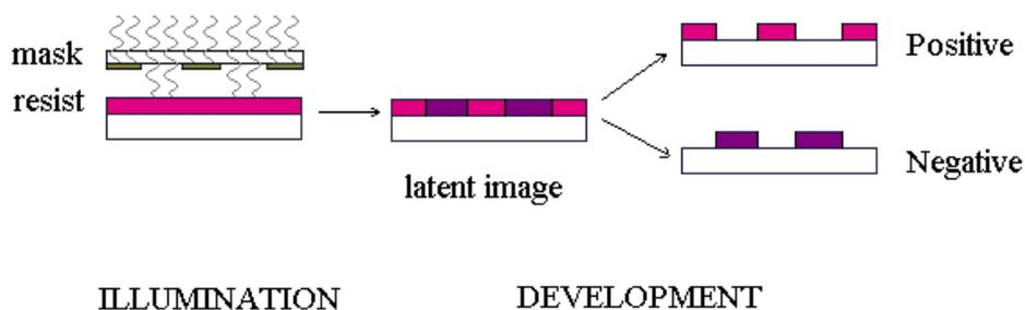
**Figure 1.** In photolithography, a surface covered with resist is illuminated through a mask and developed.
