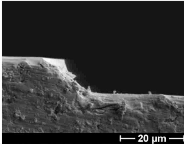
**Figure 7.** Scanning electron micrograph of cut quartz etched in BHF and sputtered with a thin ( $<0.5 \mu\text{m}$ ) film of gold. Sharp flakes are remnants of cross-section sawing.
