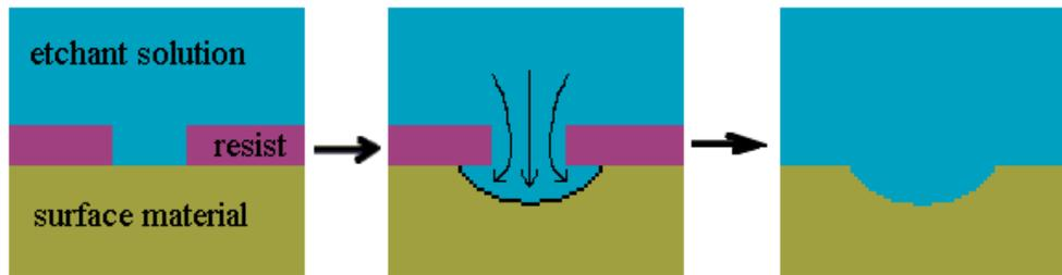
**Figure 2.** In isotropic wet etching, the material is removed equally fast in all directions and smoothly rounded edges are obtained.
