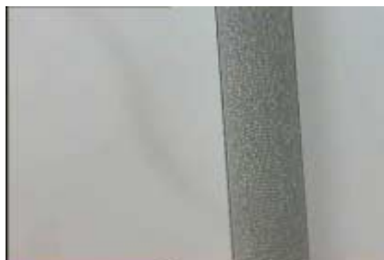
Figure 12 Milled channel with width 200 μm in PMMA.
