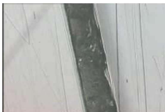
Figure 10 Milled channel with width 200 \mu\text{m} in PC.
