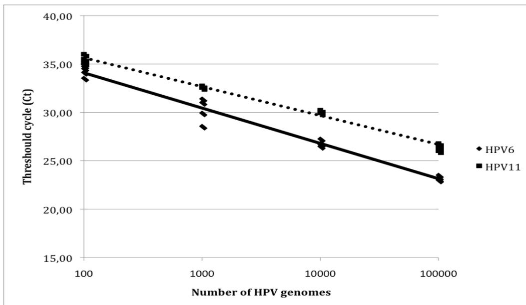
**Figure 10. HPV6 and HPV11 standard curve compared to each other.** The number of HPV genomes is plotted against threshold cycle ( $C_t$ ) number. Each dot represents a replicate of the diluted copy number of HPV genome.
