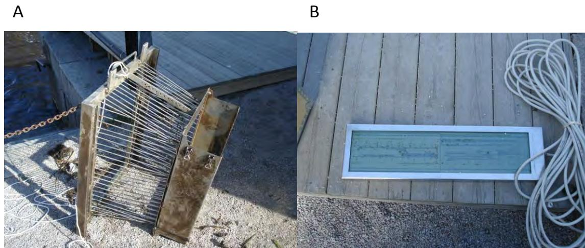
Figure 2. The slide box where the two scan plates are placed (A). One of two scan plates with IR-transmitters (B).
