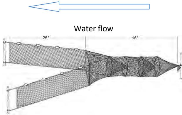
Figure 1. The fyke net used in the study was 7,5 m long, with a height of 0,65 m and a 5 m wide opening. Two nets were attached to each side of the opening with a length of 5 m.
