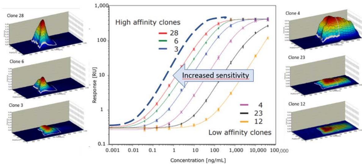
**Figure 1:** Standard curves for an immunoassay using different antibody reagents. The curve with improved sensitivity for next generation is presented as a dashed curve. Column profiles show the response signal generated for each detection antibody reagent.
