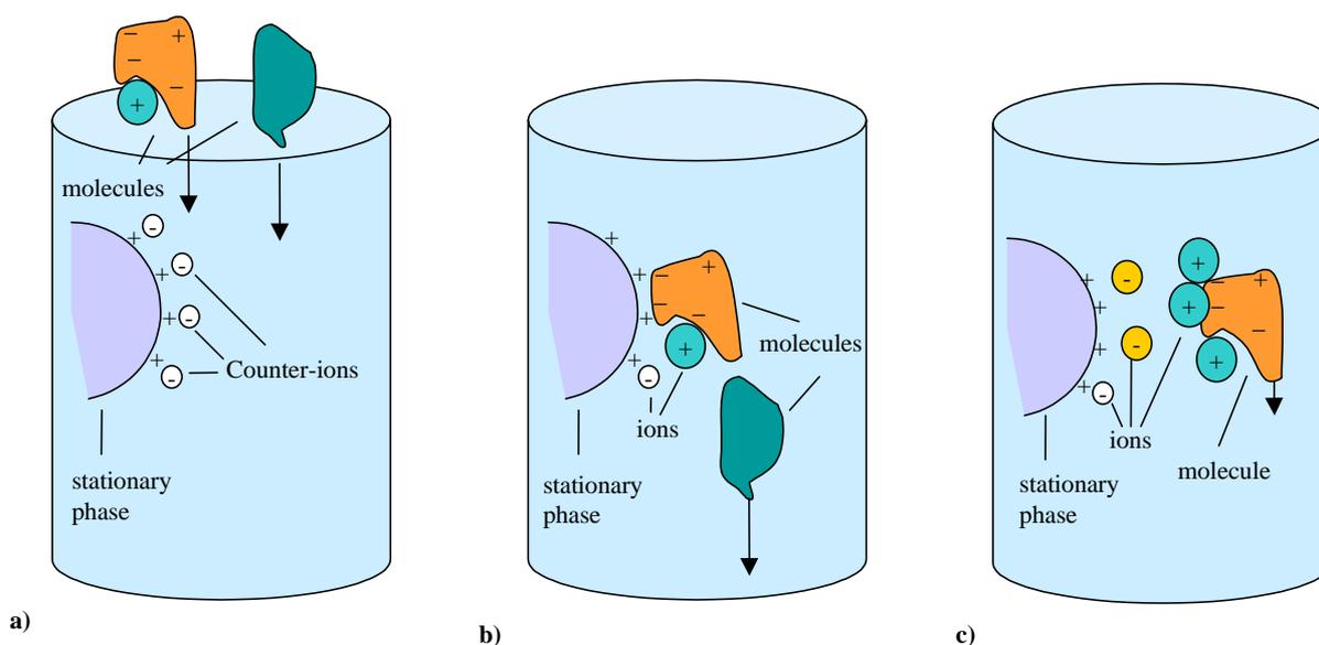
**Figure 3. A schematic picture of an anion exchange column:** *a) the charged ligands interact with counter-ions before the sample is injected. b) when only a few ions are present, the charges of the molecule interact strongly with the charged ligands on the stationary phase, causing retention or binding. c) higher ionic strength in the buffer shields the charges on both the stationary phase and charged molecules, causing weaker interactions and finally elution.*
