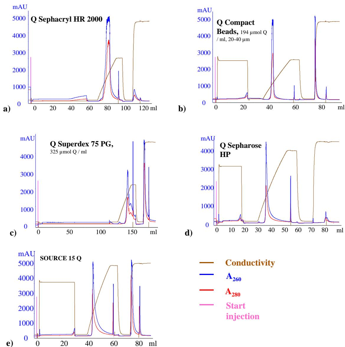
**Figure 17. Examples of chromatograms from the different media, which have been tested in this study.** The chromatograms illustrate the conductivity as well as the 260 nm and 280 nm absorbance from which the capacity, yield and recovery can be calculated. In a) and c) desalted plasmid DNA sample and 1 M NaCl gradient was used. In b) the plasmid DNA was not desalted and 1M NaCl gradient was used. In d) and e) plasmid DNA was not desalted and 2 M NaCl gradient was used.
