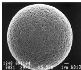
**Figure 5** Scanning electron microscopy picture of *SOURCE* bead. Illustration used with permission from Philippe Busson, Amersham Biosciences, Uppsala, Sweden.
