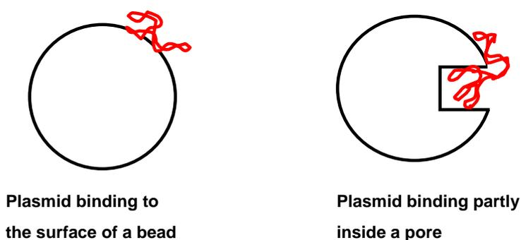
**Figure 4.** Representation of possible interactions with a chromatographic media particle and supercoiled plasmid DNA.
