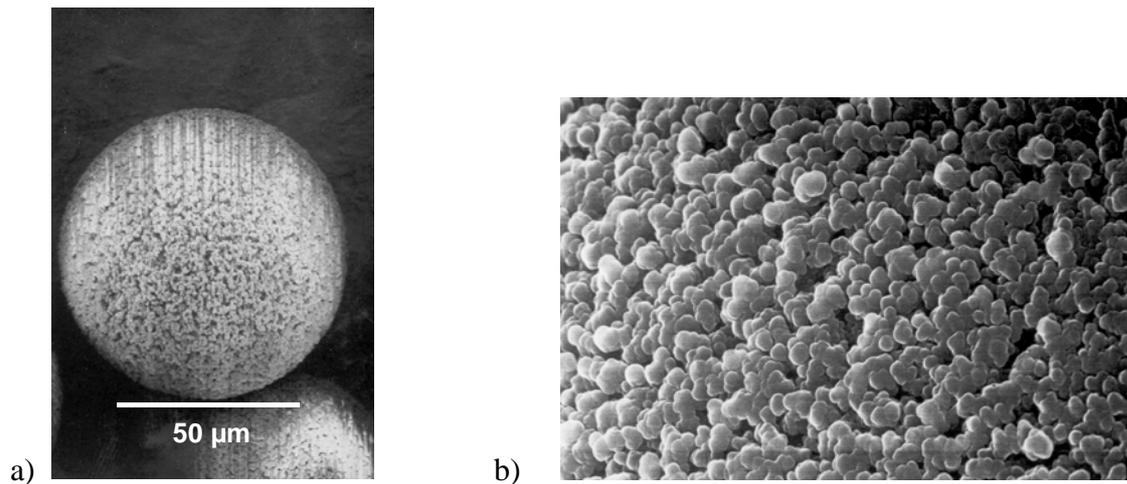
**Figure 7. Scanning electron microscopy pictures of Sephacryl 2000 High Resolution:** *a) An overview of a bead with the pores clearly visible. b) A close up on the surface of a bead. Illustration used with permission from Dag Lindström, Amersham Biosciences, Uppsala, Sweden.*
