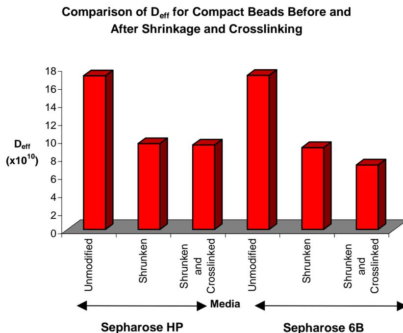
**Figure 13.** The diagram shows a decrease in  $D_{eff}$  (effective diffusion constant) after shrinkage and cross-linking of Sepharose beads. The reduced  $D_{eff}$  indicates a decreased porosity.
