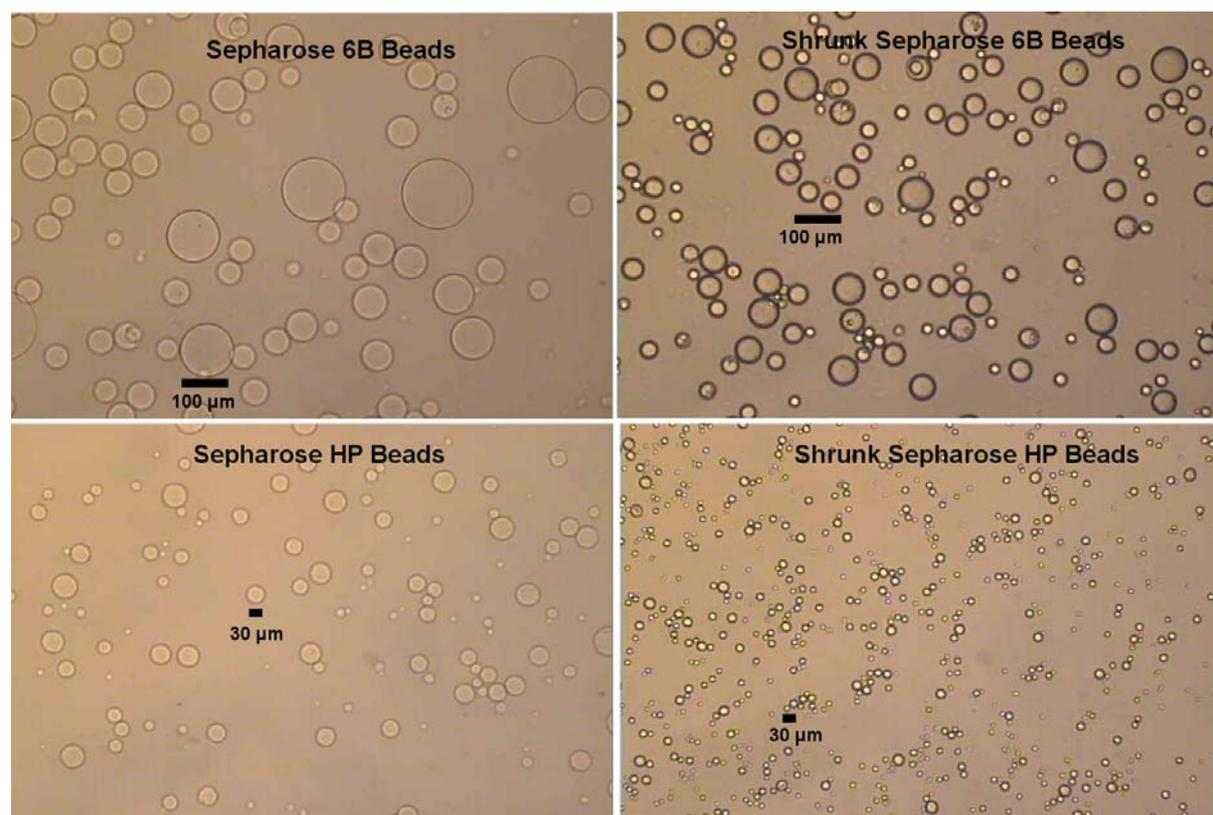
**Figure 12.** Microscopy pictures of Sepharose beads before and after shrinking.
