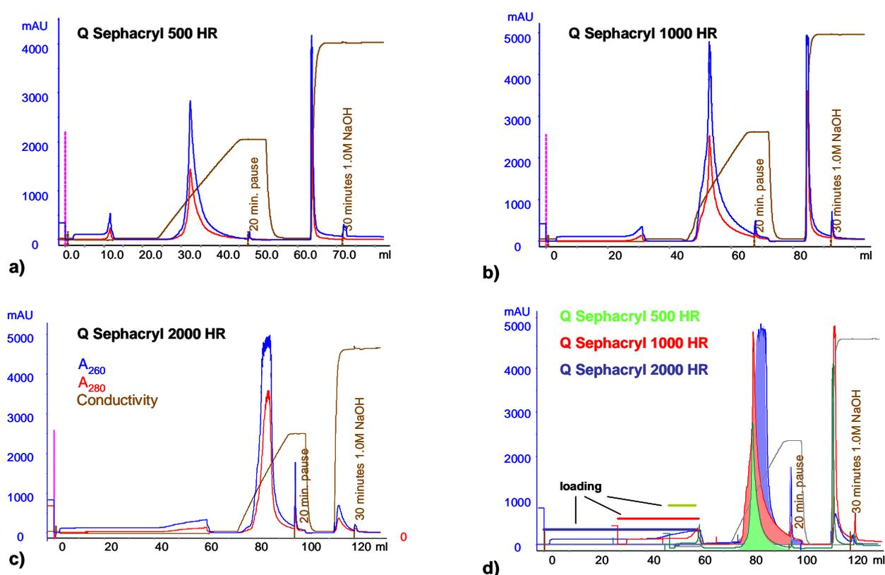
**Figure 15. Comparison of the chromatograms from the three Q Sephacryl High Resolution media:** a) chromatogram from a run on Q Sephacryl 500 High Resolution media. b) chromatogram from a run on Q Sephacryl 1000 High Resolution media. c) chromatogram from a run on Q Sephacryl 2000 High Resolution media. d) overlay of the three different peaks from the different media showing the peaks difference in peak tailing and amount of loaded plasmid DNA sample.
