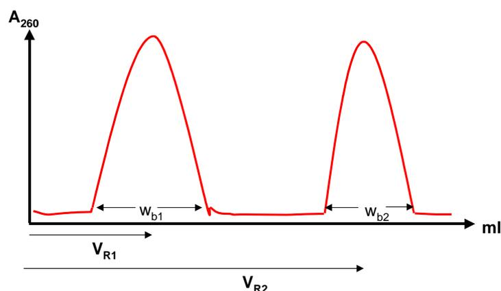
**Figure 9.** Peak widths and retention volumes for definition of resolution.
