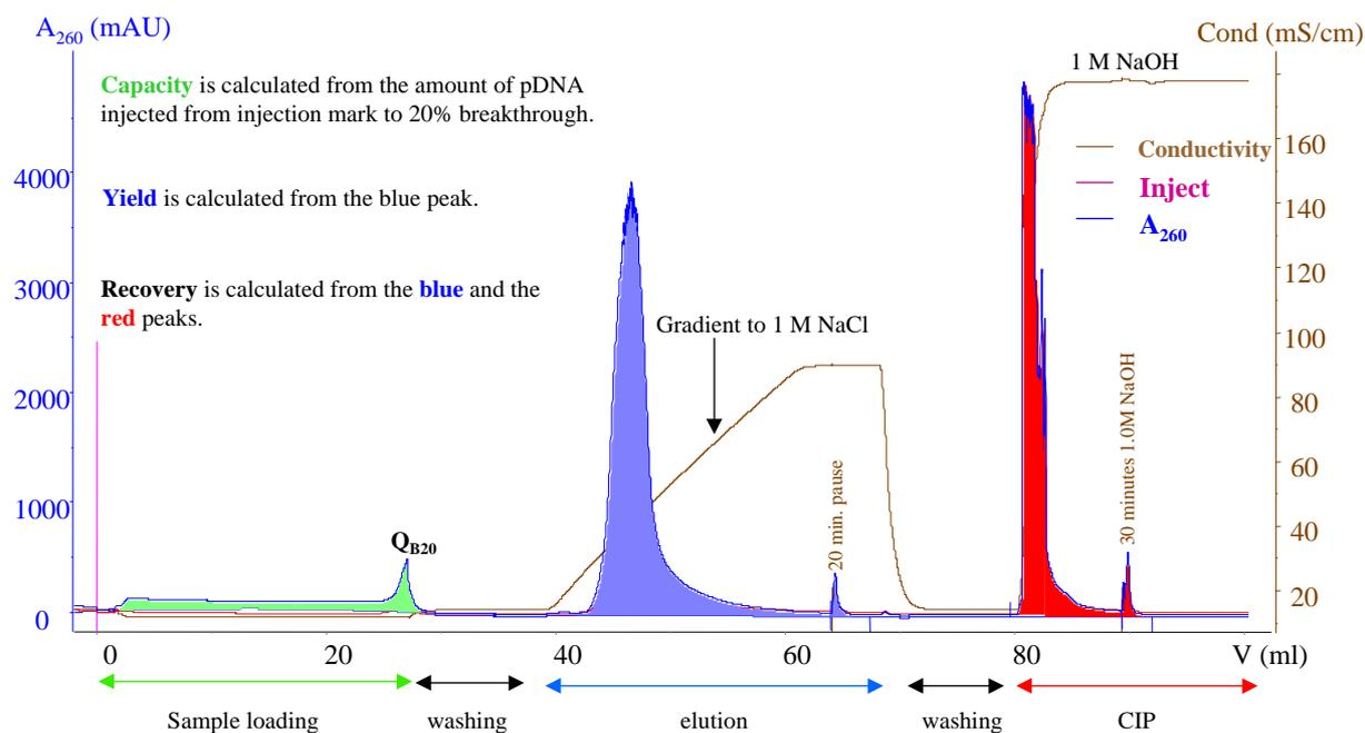
**Figure 11.** An example of a chromatogram with NaCl elution gradient and 1M NaOH CIP as well as description of capacity, yield and recovery.
