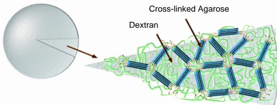
**Figure 8.** *The dextran chains are covalently linked to highly cross-linked agarose matrix. The figure shows a schematic picture of a section through a Superdex particle. Illustration used with permission from Amersham Biosciences, Uppsala, Sweden.*
