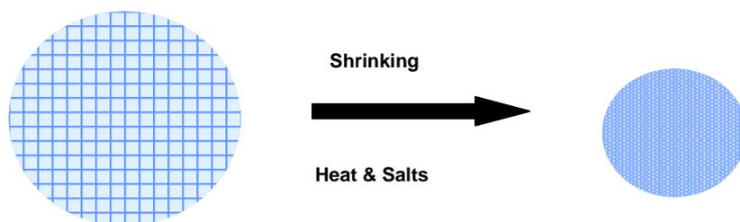
**Figure 6.** Schematic figure of the synthesis of Compact Beads, showing the smaller and more dense bead after shrinking.
