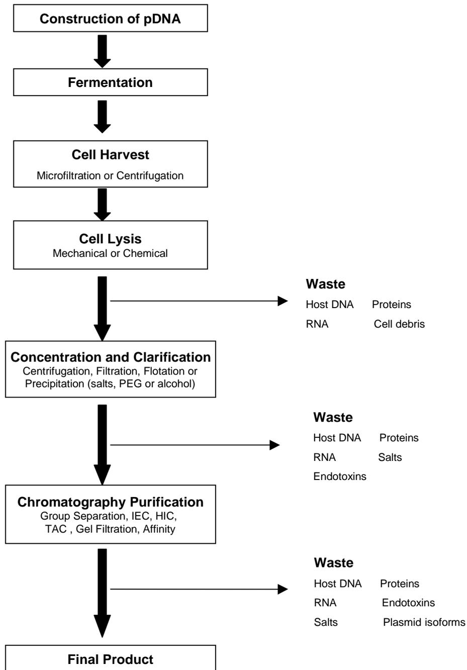
**Figure 2.** Example of a process flow sheet for plasmid DNA purification. The unit operations as well as eliminated impurities are indicated.
